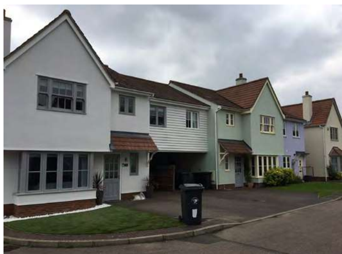
▲ Use of coloured render, jettying and varied roof forms in Hallfield, Quendon.
