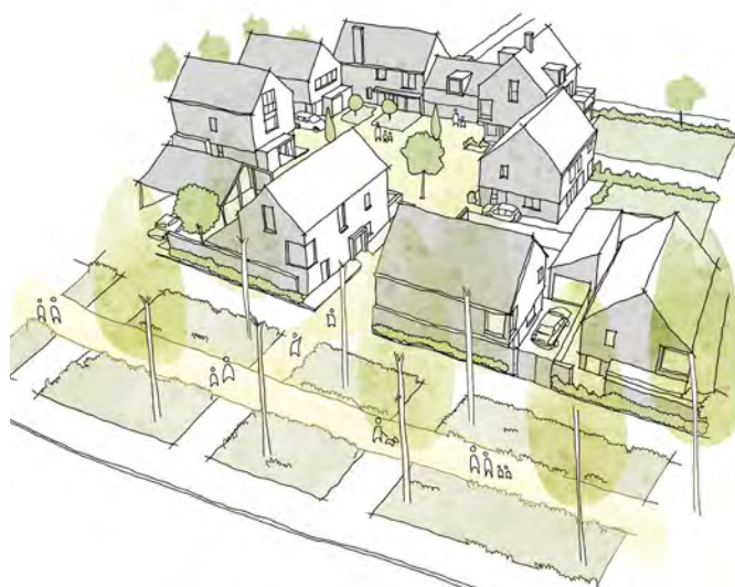
▲ Farmsteads across Uttlesford have been reinterpreted at The Avenue in Saffron Walden. The grouping utilises a local spatial typology whilst providing a mix of building types and forms. The block depth allows for efficient and interesting use of land, allowing a mature avenue of line trees to be retained.
